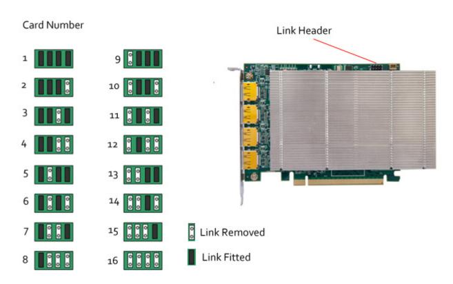
The links control the order in which the display driver uses the ImageDP4 cards. Knowing the order in which the ImageDP4 cards are used is useful when connecting the screens and the outputs from video switches.
